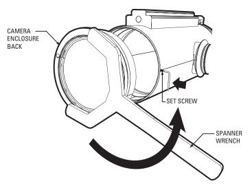
Figure 13. Remove Back Cap of Camera Enclosure
